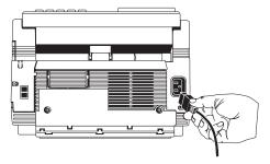
3. Connect the unattached end of the power cable into an earthed AC power outlet.
